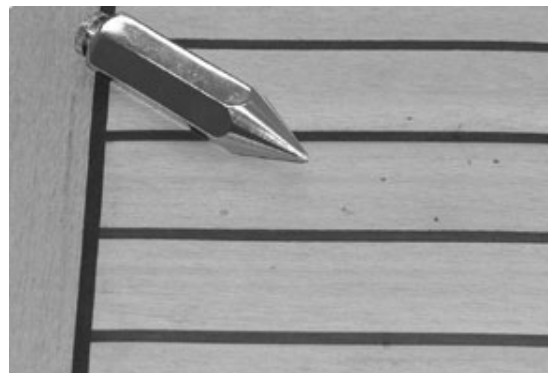
Our testing included dropping blunt objects—like this plumb bob—from above to see what damage the synthetics sustained. This Flexiteek sample was very resilient.
